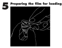
Take hold of the cassette and your end cap remover and turn out the light. Lever the cap off the cassette, and slide the film spool part way out. Find the film's shaped leader, slot this through the light-trap opening, then slide the spool back. This saves having 1.4m/4ft 8in of loose film falling on the floor.
