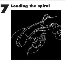
Pick up the spiral and find the projecting lugs which mark the film entry point.
