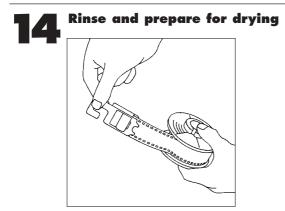
Add 5ml/l (1+200) of ILFOTOL wetting agent to the final rinse water, stir briefly, then lift the film spiral out of the tank. Pull the end of the film out of the spiral, and securely attach a wooden or plastic film clip to it.(To get a tight grip you may have to double over the end of the film.)
