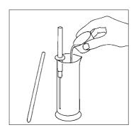
To process one 35mm film, mix the developer. Pour exactly 60ml of ILFOTEC DD–X into a measuring cup. The dilution needed is 1+4, so pour 240ml of water into a large (600ml size) cylinder. Mix hot and cold so the water is at about 23°C/73°F. Pour the developer into the water, stir with a stirring rod, and measure the temperature of the solution.
