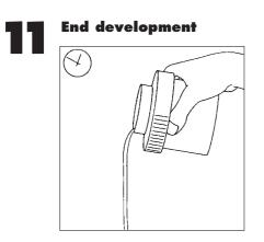
100 DELTA PROFESSIONAL film needs 12 minutes in ILFOTEC DD-X (1+4) at 20°C/68°F. Therefore, 15 seconds before the 12 minute mark is reached, start to pour the developer out of the tank.
