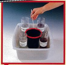
Put the bottles containing your processing solutions in a bowl of water at 40°C (104°F) 2 hours before you want to start processing. Keep an eye on the temperature if you don't have a thermostatic heater, and top the water up if it drops below 38°C (100°F).
