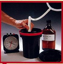
Wash the film thoroughly in running water for at least 4min.
