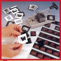
When the film is dry, cut it into individual frames and fit into slide mounts. There is a variety of mounts on the market, including plastic, glass, cardboard, masking and pin-registered mounts. Most photo libraries prefer plastic or cardboard mounts.
