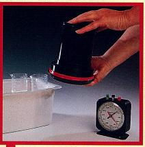
Then pour the bleach-fix solution into the tank. Invert the tank over and back for the first 15sec, then twice every 30sec for the remainder of the 10min bleach-fix stage. At the end of this time, simply pour the solution back into its bottle.
