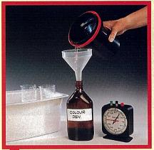
Drain water from the tank and pour in the colour developer as quickly as possible. Agitate in the same way as for the first developer. The full colour development time is 6min. About 15sec before this time is up, begin to pour the colour developer back into its bottle.
