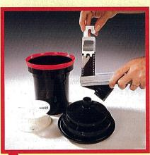
Finally, remove the film from the tank. At this point you must squeegee surplus stabiliser from the surfaces, and then hang the film up to dry. Note that while the film is wet it has an opalescent appearance – don't worry, this clears as the film dries.
