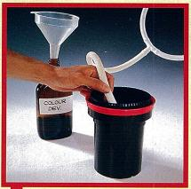
Wash for 2min in running water – again check the temperature to ensure that it is between 33-39°C. Alternatively, you can wash in four changes of fresh water. Once again, if you decide to do the latter, it is important to agitate each change for ½min.
